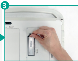
3 Pull the tape on the top of the SSD door to loosen the SSD.
