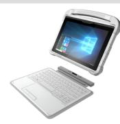
2 Fold the kickstand and keyboard toward the 301MD tablet for portability and as a protective cover to shield the screen.
