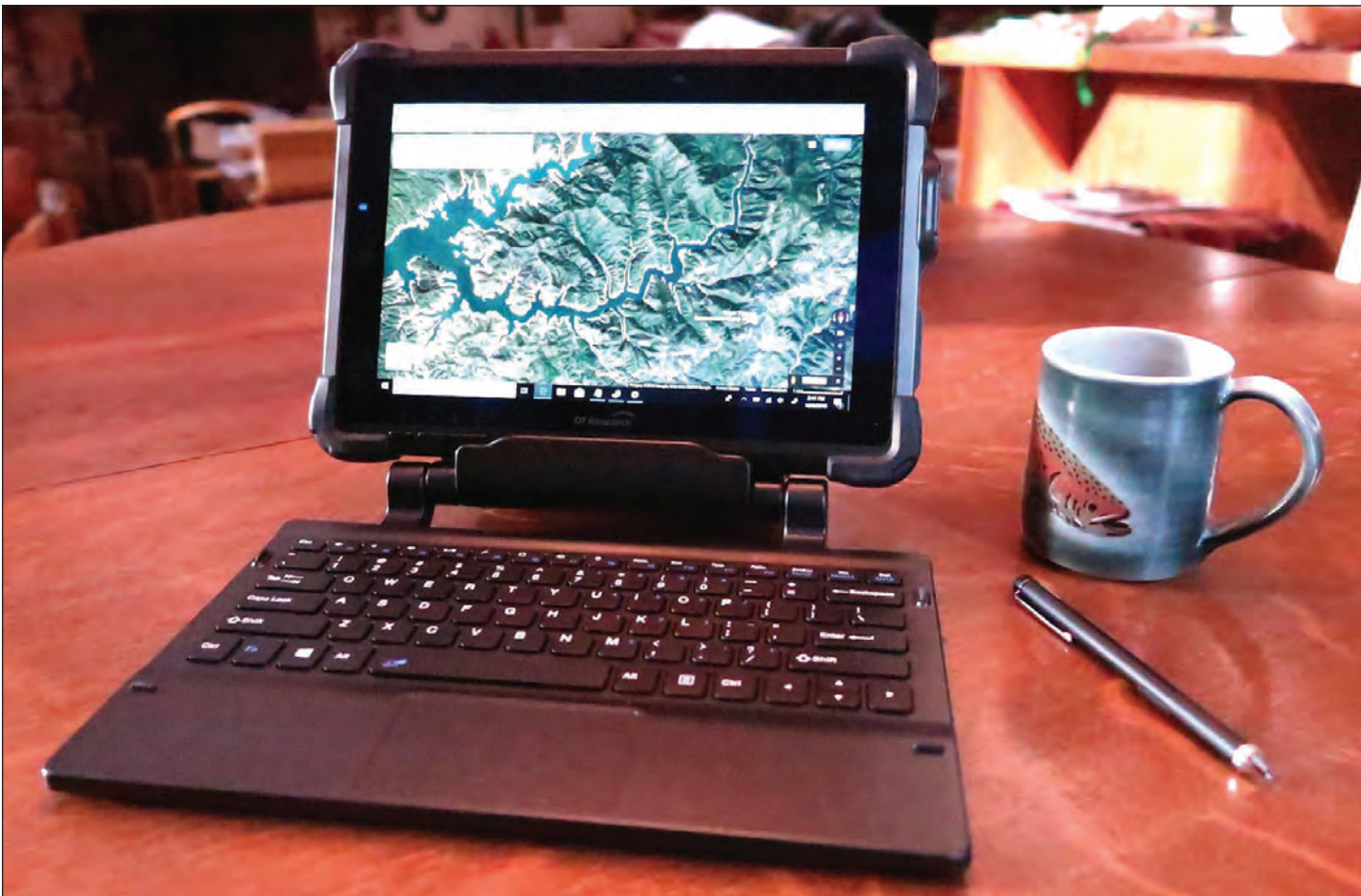
An optional keyboard connects easily to the DT301T Rugged RTK Tablet. Photo by Steve Wilent.
