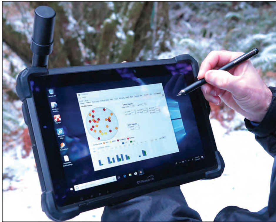
Figure 1. DT Research’s DT301T Rugged RTK Tablet with the detachable Harxon GNSS antenna. Photo by Steve Wilent.
