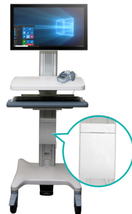
12V DC-output powers mobile printer
