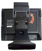
Remove the detachable base by pressing upward to remove the cover, then unscrewing the four screws attaching the base to the display.
