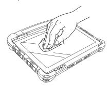
2 Use the included dust-absorber to remove dust
