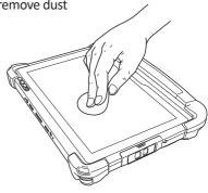
4 Carefully align one edge of the film to the corresponding one of the screen, then apply the film onto the screen
