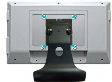
2. Attach the stand to the display. Screw the VESA-compliant bracket of the stand to the display with four (4) screws.
