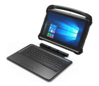
2 Fold the kickstand and keyboard toward the DT311Y tablet for portability and as a protective cover to shield the screen.
