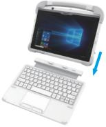
2 Fold the kickstand and keyboard toward the DT301Y, DT301YR or 301Y/MD tablet for portability and as a protective cover to shield the screen.
