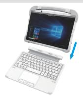
2 Fold the kickstand and keyboard toward the DT301Y, DT301YR or 301Y/MD tablet for portability and as a protective cover to shield the screen.
