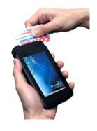
The DT433SC/SQ has a large and easy-to-read screen and hot-swappable battery, making data access efficient and optimizing staff workflow.
